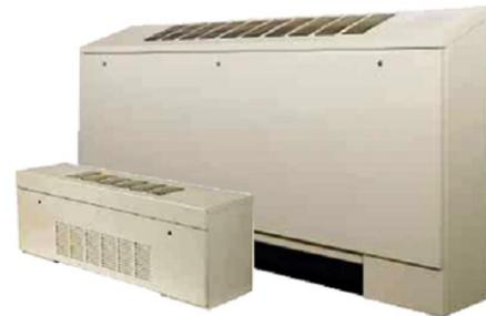
The EC motor used is specifically designed with fan coil horsepower requirements in mind (less than or equal to 1/4 HP). The new fan coil EC motors operate in a constant RPM mode compared to a constant airflow mode often associated with EC motor technology applied in Variable Air Volume boxes. Constant airflow applied in a fan coil application reduces efficiency.
